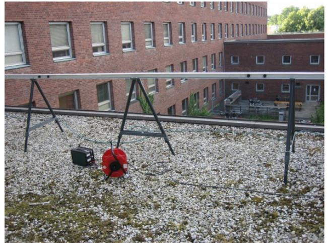
FIGURE 8. Antenna array used for measurements.
