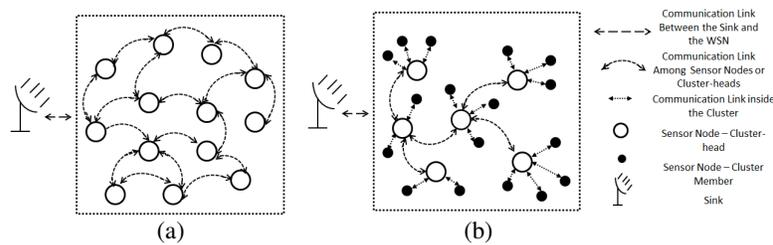
**Fig.1.** WSN architectures: (a) Planar; (b) Hierarchical.
