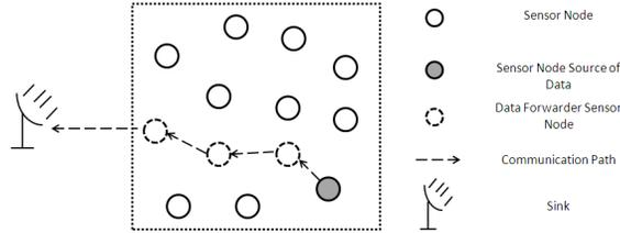
**Fig.2.** Multi-hop data communication from a data source sensor node towards the sink.
