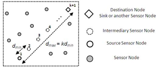
**Fig.3.** Distances between communicating nodes and intermediary nodes.
