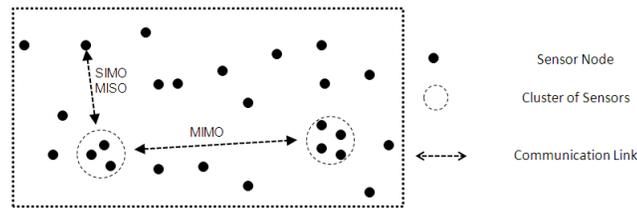
**Fig. 4.** Cooperative MIMO communication between clusters of sensors and SIMO/MISO communication between a cluster and an individual sensor.
