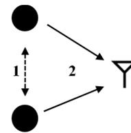
Figure 4. Example of a  $2 \times 1$  MISO system.
