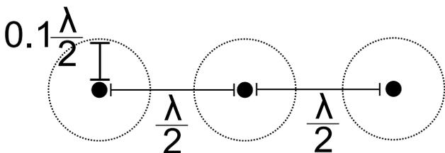
Figure 6: Graphical example of antenna displacement
