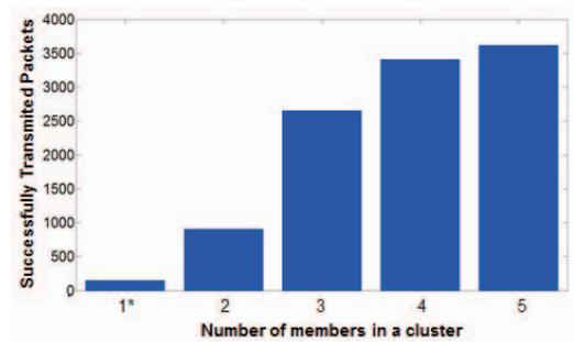
Figure 11. Successfully transmissions at 15s transmission time.
