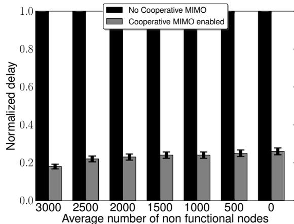
Figure 7: Normalized packet delivery delay comparison between cooperative MIMO networks and non cooperative MIMO networks
