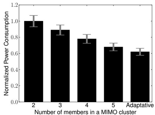
Figure 8: Energy consumption comparison between different cooperative MIMO configurations with fixed number of cluster members and the proposed adaptive algorithm.
