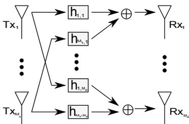
Figure 1: Example of a  $Q$  by  $Q$  MIMO system
