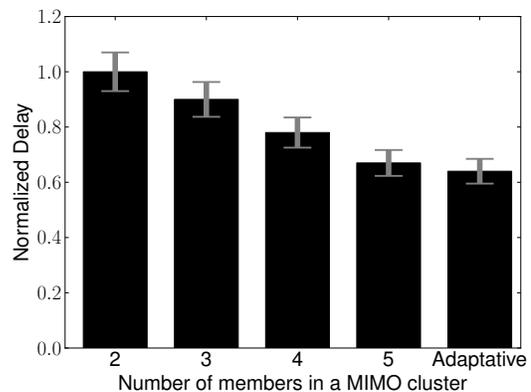
Figure 9: Delay comparison between different cooperative MIMO configurations with fixed number of cluster members and the proposed adaptive algorithm.
