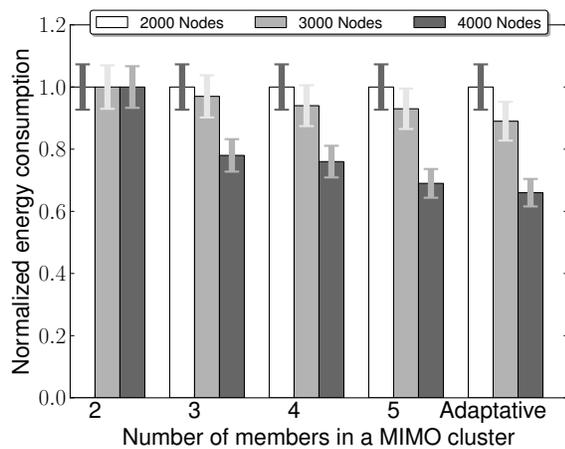
Figure 10: Energy consumption comparison between different MIMO cluster configurations and number of nodes active in the area.
