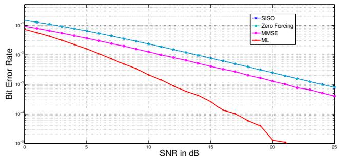
Figure 2: Performance comparison between standard SISO systems and  $2 \times 2$  MIMO systems using Zero Forcing, MMSE and ML equalization
