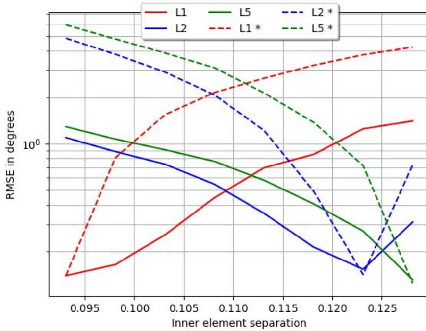
**Figure 2:** Direction of arrival estimation performance for multiple frequency bands versus inner element separation in meters
