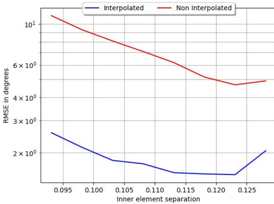
**Figure 3:** Combined direction of arrival estimation performance versus inner element separation in meters
