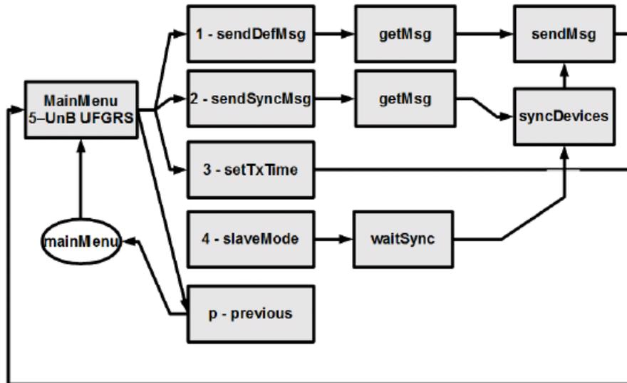
Fig. 4. Block Diagram of the Developed Firmware.
