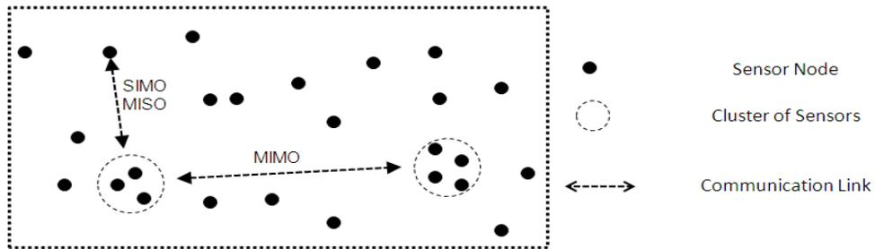
**Fig. 1.** Cooperative MIMO Applied to WSN: communication between clusters of sensors nodes and SIMO/MISO communication between a cluster an individual sensor.
